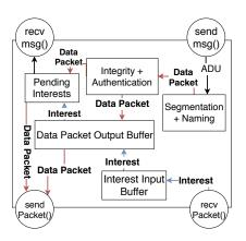
**Figure 2: Producer socket**
